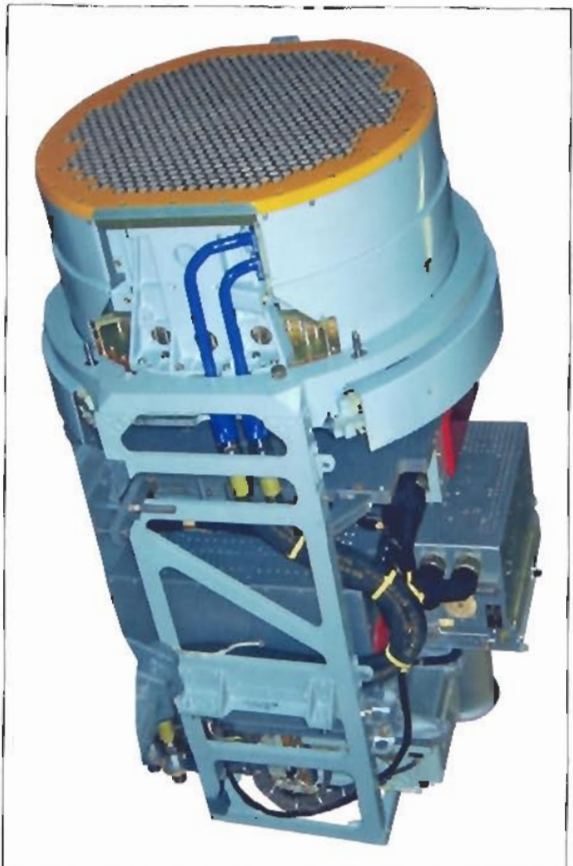
First model of active-phased-array radar (Zhuk-ME)
